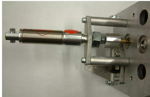
Step 3: Thread the 5/8-16 nut onto the cylinder nose. Tighten the 1/4-28 nut against the shift block.
